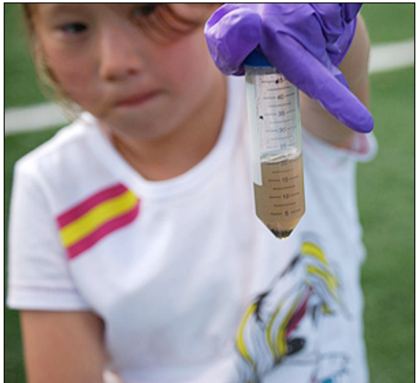
A water sample from artificial turf contains particles of the crumb rubber used as fill to keep the plastic blades upright.
